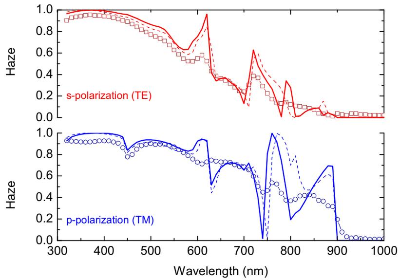
Figure 8: Haze of the 260 nm thick a-Si film on the textured silver reflector (same as Figure 5). Dashed and full lines denote theoretical results for conformal and non-conformal covering, respectively, using an expansion to third order and the data of bulk silver.
