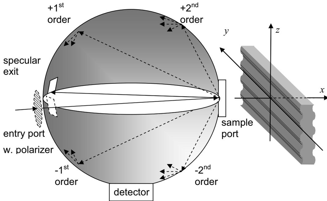
Figure 1: Configuration of the measurement geometry in the integrating sphere. Incident and reflected beams span the horizontal plane, diffracted beams propagate upwards and downwards; the latter can hit the detector before being randomized.
