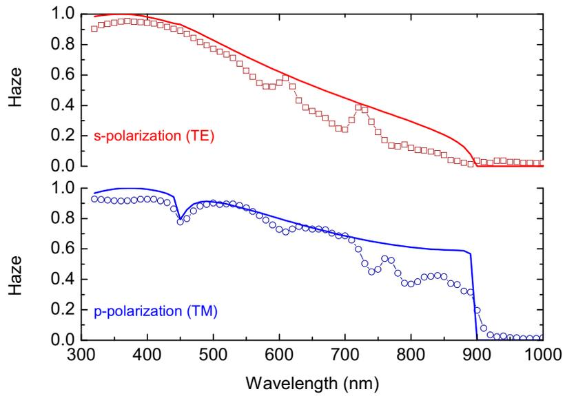
Figure 5: Measured haze from a 260 nm thick a-Si film on the grating; squares and circles represent s- and p-polarization, respectively. The solid line shows the calculated haze for reflection from corrugated bulk a-Si.
