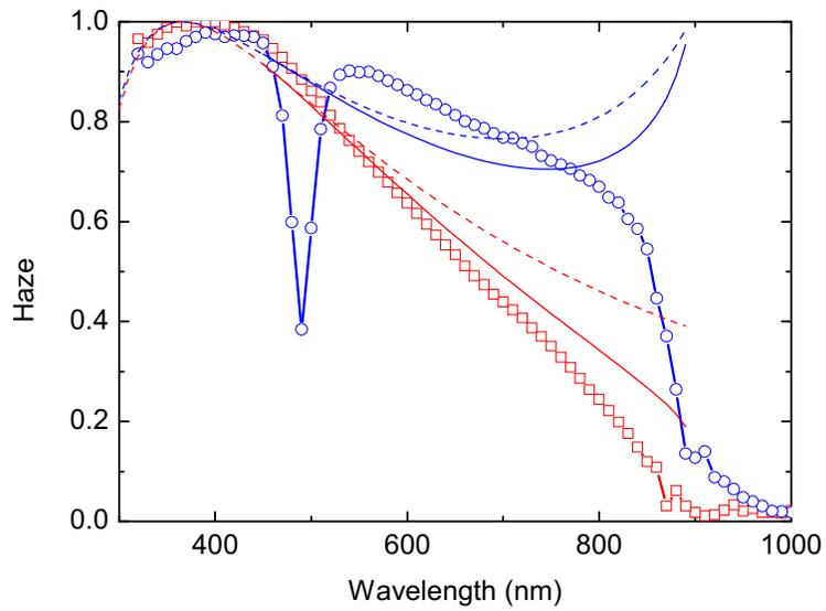
Figure 3: Measured reflection haze of a sinusoidally textured silver surface with period of 890 nm for perpendicular incidence with s- (squares) and p-polarized light (circles). Dashed and full lines represent results of scalar scattering theory before and after correction for the effective depth of the texture, respectively.
