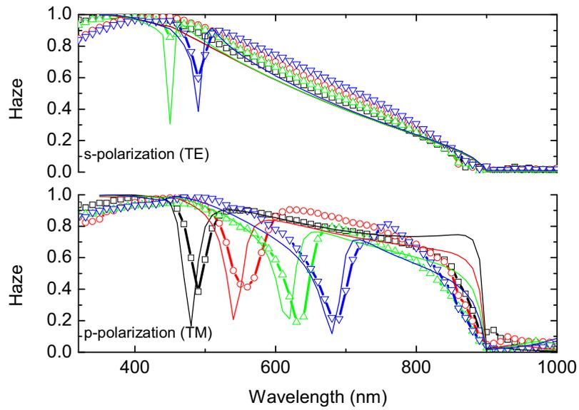
Figure 6: Haze of the sinusoidal silver surface covered with thin films of ZnO; squares reproduce the properties of the pure silver surface from Figure 3, circles, up-, and down triangles denote film thicknesses of 20, 40, and 60 nm, respectively. The overlaid lines illustrate theoretical results for expansion to third order.
