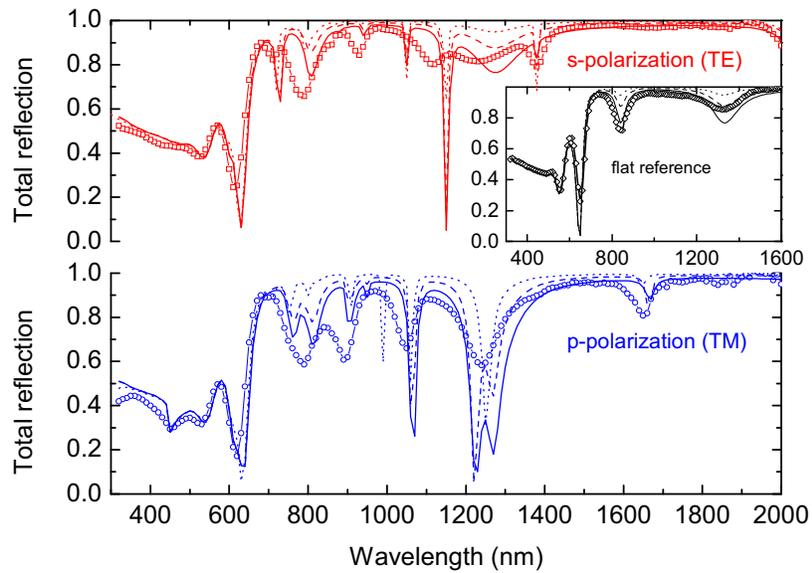
Figure 7: Total reflection of a 260 nm thick film of a-Si on the textured silver reflector; squares and circles denote p- and s-polarization, respectively. In the inset, diamonds illustrate the reflection from a flat reference sample. In all panels, the lines show theoretical results for expansion to third order using the dielectric data of bulk silver (dots) and two models of silver with reduced material quality (dashed and full lines).
