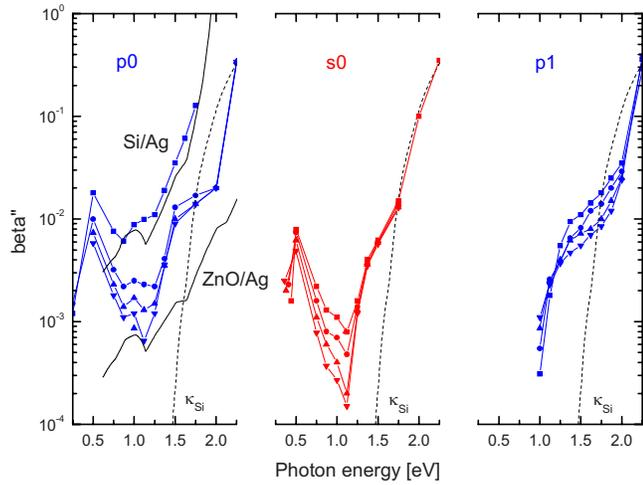
FIG. 7. (Color online) Imaginary part  $\beta''(\omega)$  of the lowest order guided modes in Fig. 6. The dashed line represents the extinction coefficient of silicon ( $\kappa_{\text{Si}}$ ) and the full lines in the left panel denote the normalized attenuation of the plasmon dispersion relations of the Si/Ag and the ZnO/Ag interfaces according to Eq. (4). Squares, circles, up and down triangles correspond to ZnO thickness of 0, 20, 40, and 60 nm, respectively.
