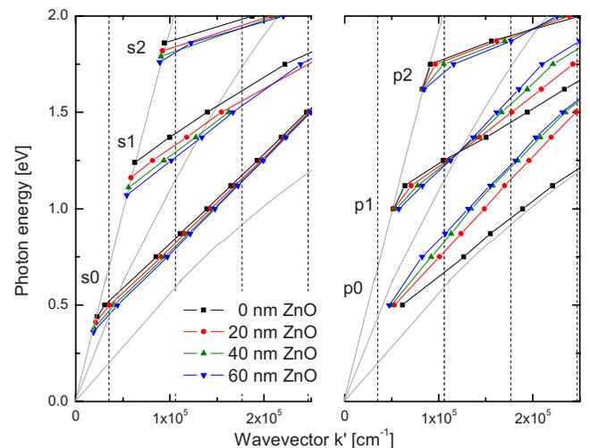
FIG. 4. (Color online) Calculated dispersion relations  $\omega(k)$  for the configurations shown in Fig. 3, using the same symbol types and scale. Different from the measurement on the sinusoidal grating, the flat interface model predicts higher energies for all  $p0$  modes.
