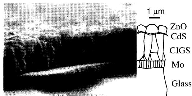
Figure 3: Cross section image of a CIGS solar cell. The different layers are clearly distinguished; molybdenum at the bottom with very small grains, vertical structures of the absorber and flat grains on the top which make the front contact.
